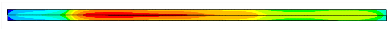
Temperature distribution in Target for P=750 kW (Graphite thermal conductivity= 35 W/m/K, H = 450 W/m 2 /K)
